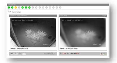
You are alerted if cameras have been tampered with, obscured, are out of focus, or too bright or dark.
